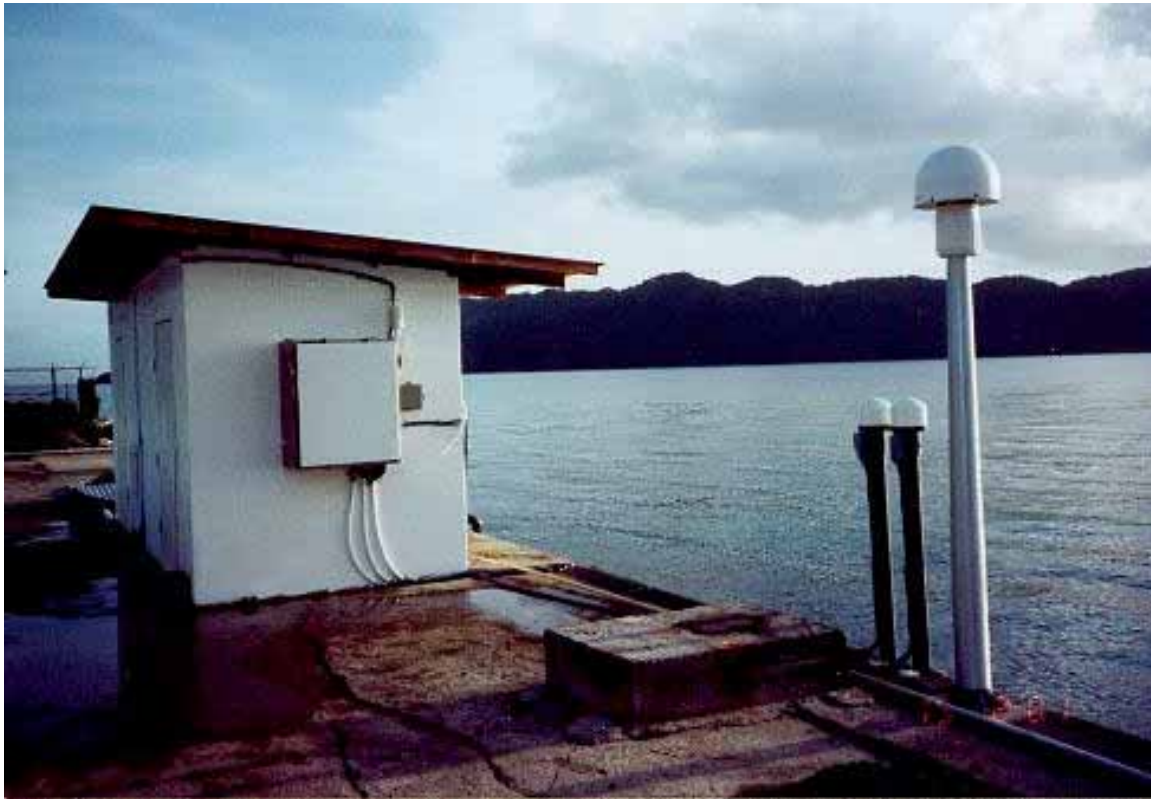
Figure 4. University of Hawaii tide gauge at Palau showing twin Aquatrak acoustic gauges, CGPS receiver, and instrument hut.
